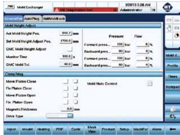
Integrated one-key mold exchange control for unmanned process exchange and improved productivity
