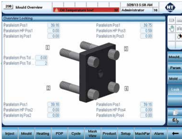
Platen parallelism monitoring for effective protection of the mold and smooth operation of the machine
