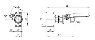
Adjustable screw joint set, scale 1:5
