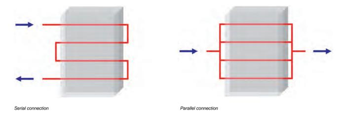
In order to take full advantage of temperature control circuits connected in parallel, it is advisable to measure and monitor the flow rates of the individual circuits.
