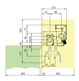
Parallel connection of two circuits, scale 1:5
