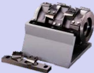
By means of the rotor setting device the rotor knives can be adjusted outside the granulator without interrupting the granulating process in units with an exchangeable rotor (optional).
